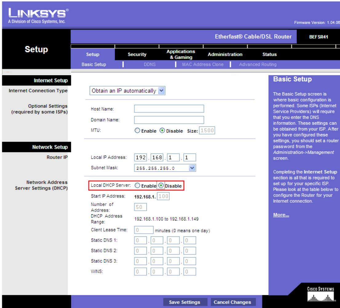
The screenshot shows the Linksys Basic Setup page for an Etherfast Cable/DSL Router (BEFSR41). The page is divided into several sections: Internet Setup, Network Setup, and Basic Setup. The Local DHCP Server setting is highlighted with a red box, showing it is currently disabled. The Start IP Address is 192.168.1.100, and the Number of Address is 50. The DHCP Address Range is 192.168.1.100 to 192.168.1.149. The Client Lease Time is 0 minutes. The Static DNS and WINS settings are all set to 0.
