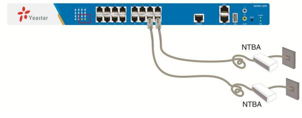
Figure 3-4 Connection of BRI ports
