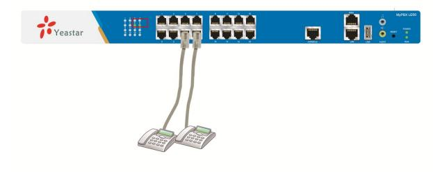
Figure 3-5 Connection of FXS ports
