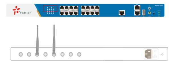
Figure 3-3 Connection of GSM/UMTS ports
